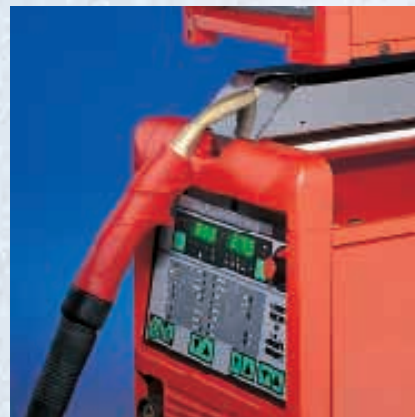
Integral torch holder on the "PickUp" trolley
