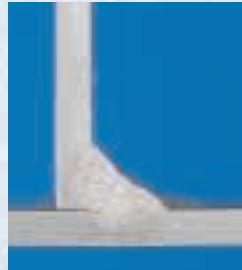
With start-up program - no fusion defects
